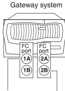
One port on each of two different cards is configured to ensure redundancy to the port pair on the storage array. Then, if one card fails, the port on the other card is used. You can use either port on a card.
